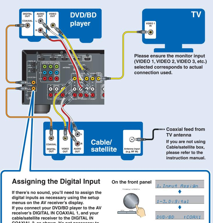
COAXIAL 2, as shown, it's not necessary to assign the digital input.
